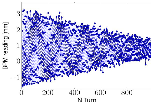
Figure 3: BPM signal,  $\beta_x=12$  m at BPM location.
