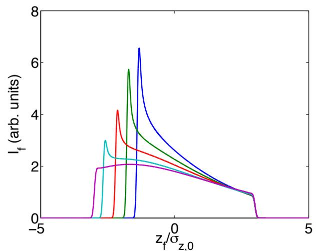
Figure 1: Current profiles analytically obtained from Eq. 3 for  $b_f = 0.7$  and  $a_f = 2.0, 2.25, 2.5, 2.75,$  and  $3.0$  corresponding to decreasing current from blue to magenta traces (we took  $\sigma_u = 0.05$ ).
