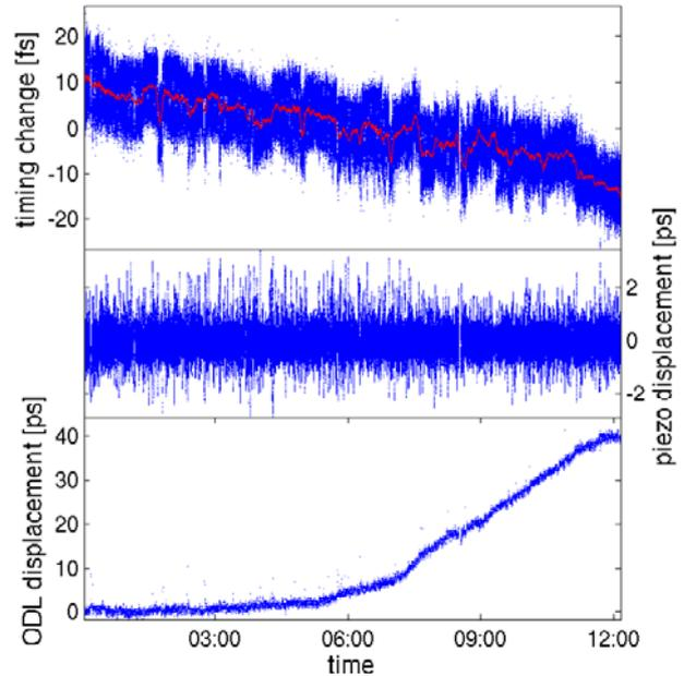
Figure 5: Out of loop drift measurement of a 400 m long fiberlink. Top: end of link timing change (blue). Over 12 hours the rms jitter is  $(7.5 \pm 1.8)$  fs with a timing drift of 25 fs. The red line indicates changes with a time constant of 100 s. The timing jitter faster than 100 s is  $(4.4 \pm 1.1)$  fs. Middle: piezo stretcher displacement. Bottom: Displacement of optical delay line (ODL).
