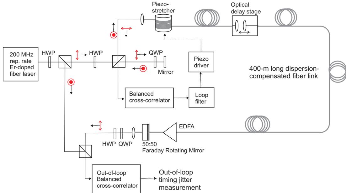
Figure 2: Experimental setup for the fiberlink stabilization.
