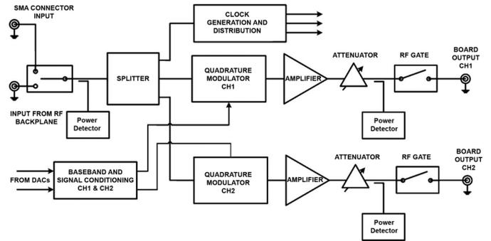
Fig. 2. Block diagram of the analog subsystem of the vector modulator card.
