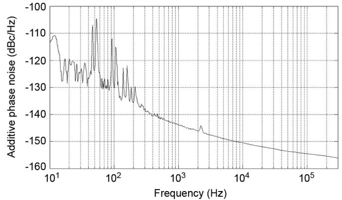
Fig. 8. Additive phase noise spectrum of the vector modulator card.
