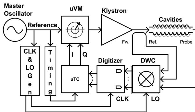
Fig. 1. LLRF system architecture. The vector modulator (uVM) is an actuator, and uTC is a controller in the feedback loop.
