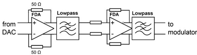
Fig. 3. Block diagram of the baseband signal conditioning chain.
