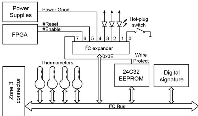
Fig. 6. Block diagram of the module management subsystem.
