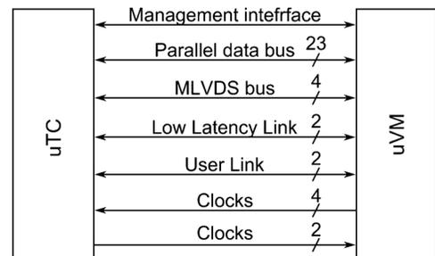
Fig. 5. uVM Zone3 interconnections block diagram.
