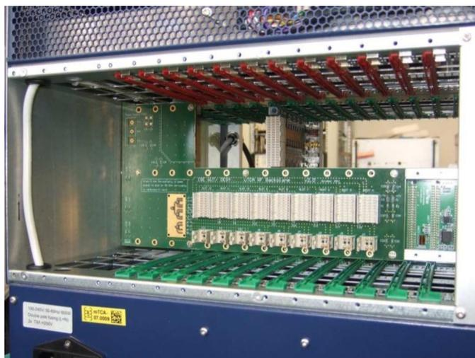
Fig. 5. RF backplane prototype assembled in the MTCA.4 crate.
