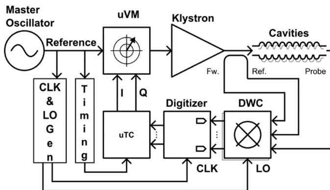
Fig. 1. LLRF system architecture and signal flow.
