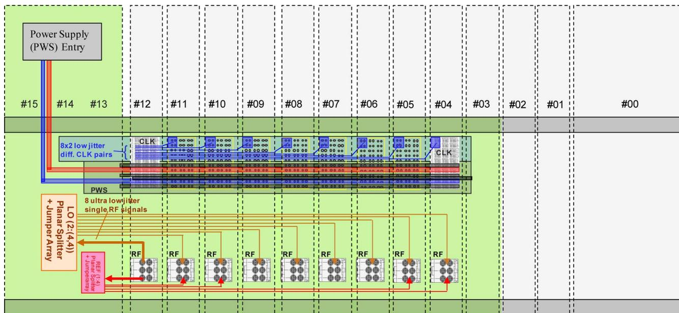
Fig. 4. RF backplane prototype block diagram.
