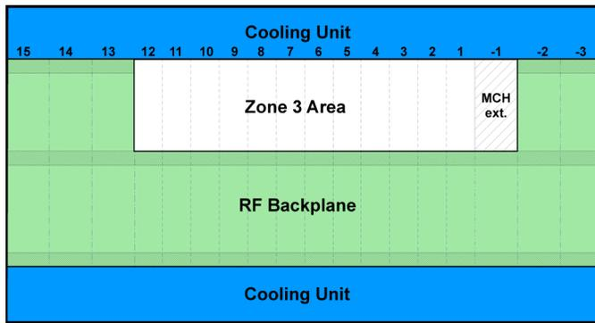
Fig. 3. Area available for  $\mu$ RFB in the MTCA.4 crate (rear view).
