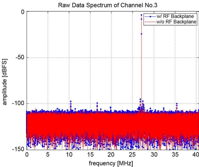
Fig. 7. Comparison of signal spectrum recorded by digitizer (AMC) supplied by the downconverter module ( $\mu$ RTM) when LO and CLK signals were provided via front panels (red) and via the  $\mu$ RFB (blue).
