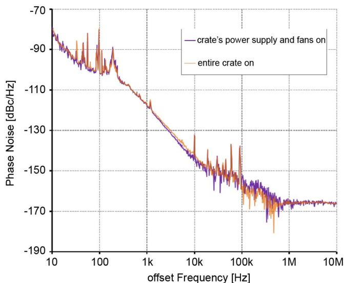
Fig. 6. Phase noise of 1.3-GHz signal distributed over the backplane inside of MTCA.4 crate equipped with fans and DSP subsystems.
