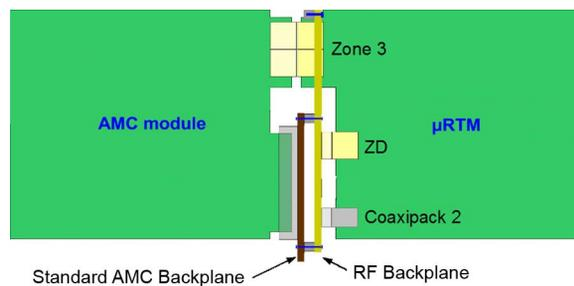
Fig. 2. RF backplane position in the MTCA crate.
