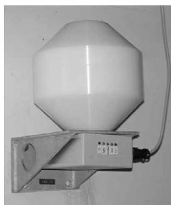
Figure 7. The wall mounted RadMon detector.
