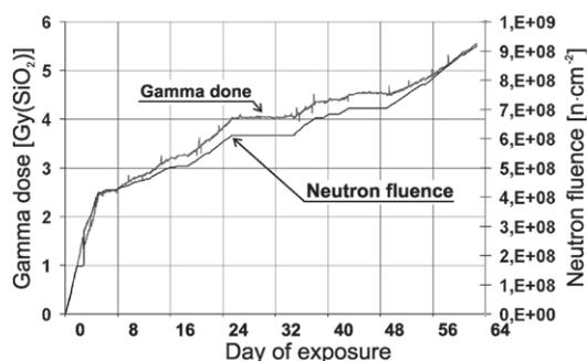
Figure 9. The accumulated dose of gamma radiation and neutron fluence registered in the FLASH.
