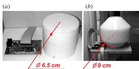
**Figure 4.** Polyethylene moderators: (a) 6.5 cm cylindrical and (b) 9 cm semi-spherical moderators.
