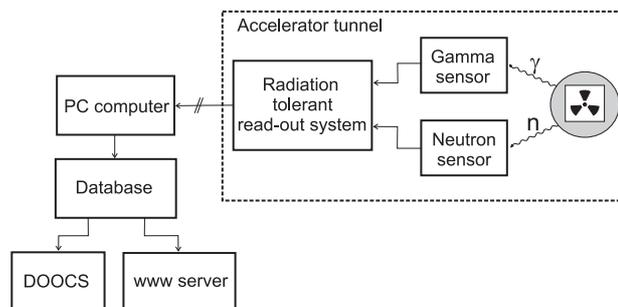
Figure 2. The block diagram of the radiation monitoring system RadMon.
