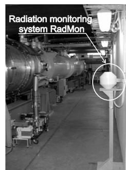
Figure 8. The portable RadMon device.
