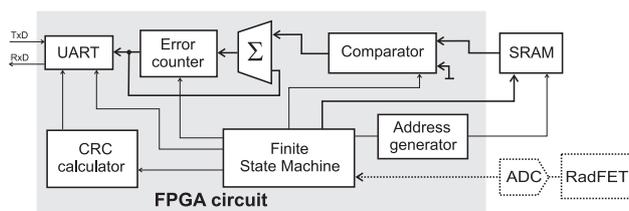
Figure 6. The block diagram of the FPGA-based RadMon.
