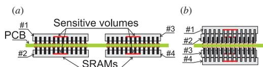
**Figure 5.** The SRAM-based sensors: (a) the flat version and (b) the sandwich structure.
