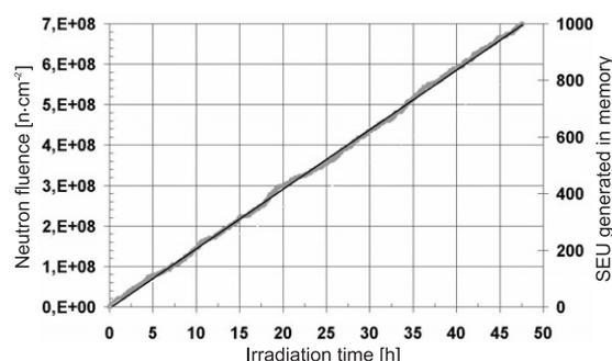
**Figure 3.** Accumulated neutron fluence and number of SEUs generated in the 512 kB memory irradiated from  $^{241}\text{AmBe}$ .
