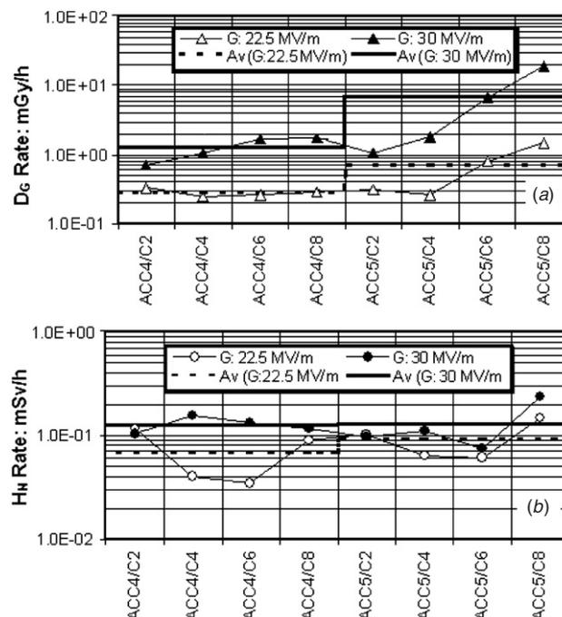
**Figure 11.** Showing (a) gamma dose rate  $D_G$  and (b) effective dose equivalent rate of neutrons  $H_N$  near accelerator modules #4 and #5 evaluated using Gaf-EBT films and bubble detectors respectively. The gradient across the modules and the average neutron and gamma dose rates are also indicated.
