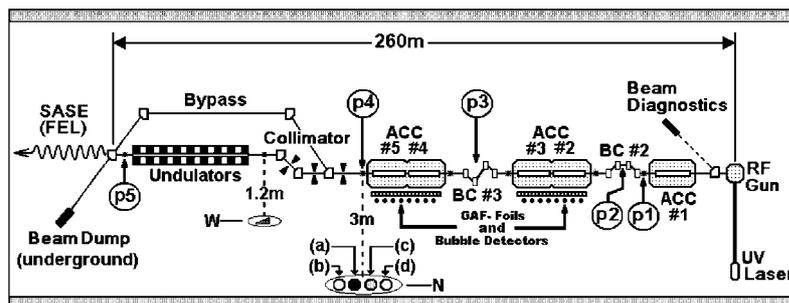
**Figure 1.** Showing the main components of the FLASH facility; p1, p2, p3 and p4 are the locations where radiation measurements were made using GaAs LED. The figure is explained in detail in the main text.
