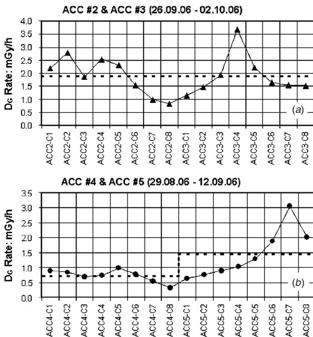
**Figure 12.** Showing the gamma dose rates  $D_G$  near the accelerator module pairs #2 and #3 (a) and #4 and #5 (b) evaluated using Gaf-EBT films during routine operation mode. The average gamma dose rates are indicated by the dotted lines. Modules #2, #3 and #5 were operating at the gradient of  $21 \text{ MV m}^{-1}$  whereas the module #4 operated at  $16 \text{ MV m}^{-1}$ .
