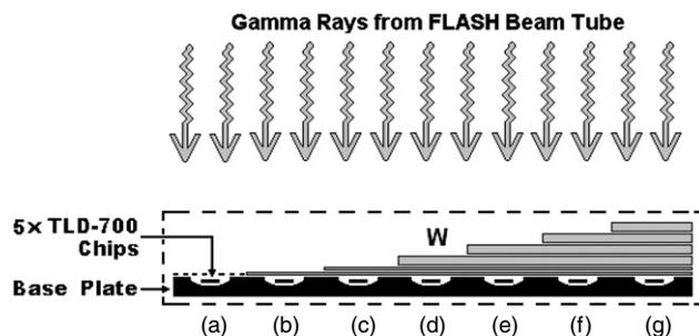
**Figure 8.** Showing the construction details of the lead attenuator wedge used for the unfolding of a bremsstrahlung spectrum at FLASH.
