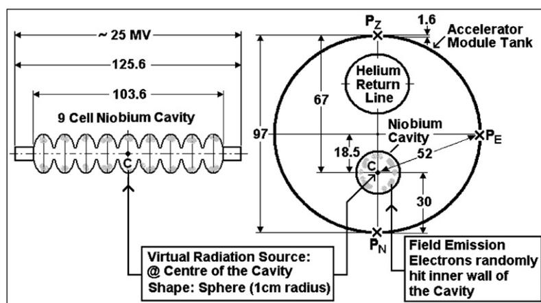
**Figure 2.** Showing the important dimensions (in centimetres) of the accelerator module tank and nine-cell niobium cavity developed on TESLA technology at DESY.
