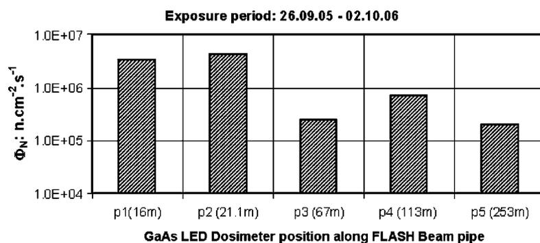
Figure 5. Neutron fluence rates at several critical locations along the FLASH beam pipe evaluated using GaAs LED dosimeters.
