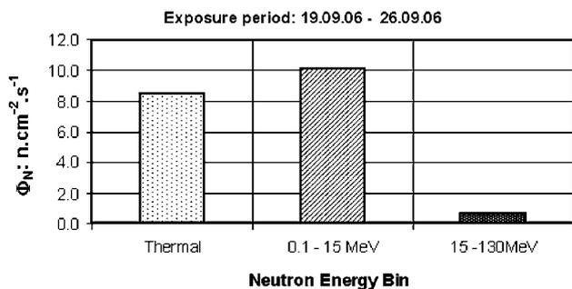
**Figure 7.** The three-bin neutron spectrum near accelerator module #5 of the FLASH evaluated using superheated emulsion (bubble) detectors.
