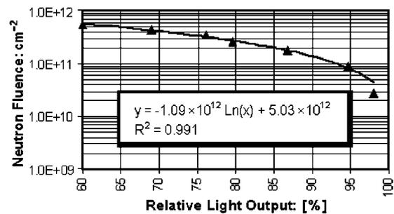
**Figure 4.** The neutron fluence (FLASH spectrum) is shown as a logarithmic function (inset) of the relative light output of the GaAs LEDs.
