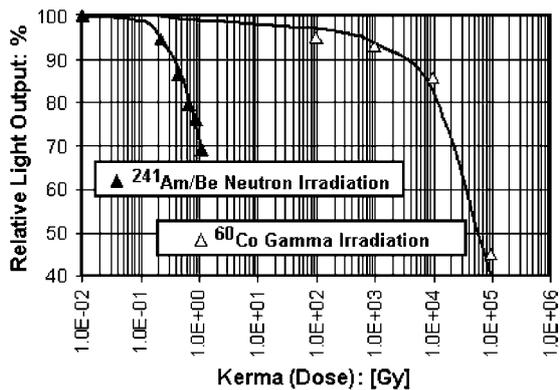
**Figure 3.** Showing the relative light output of GaAs LEDs irradiated with neutrons and photons from standard sources. The light outputs are normalized with the control (unirradiated) LEDs.
