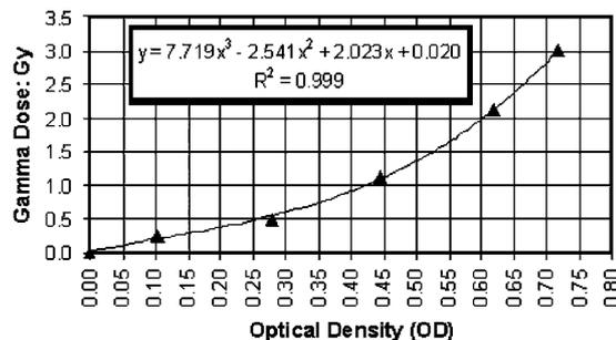
**Figure 10.** Showing the gamma dose delivered to the Gaf-EBT film as a function of optical density. The data points are fitted with the calibration polynomial (inset).
