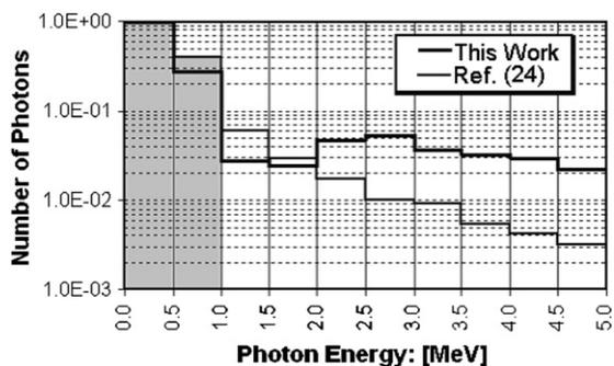
**Figure 9.** Showing the unfolded bremsstrahlung spectrum at FLASH and the computer-simulated spectrum adopted from reference.
