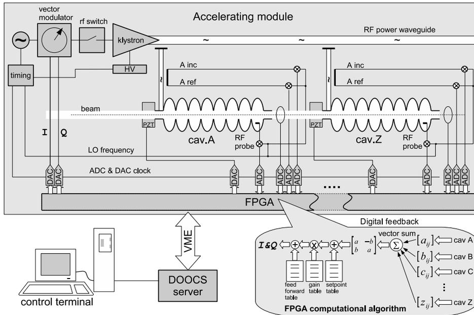
Figure 1. Architecture of a typical RF system.
