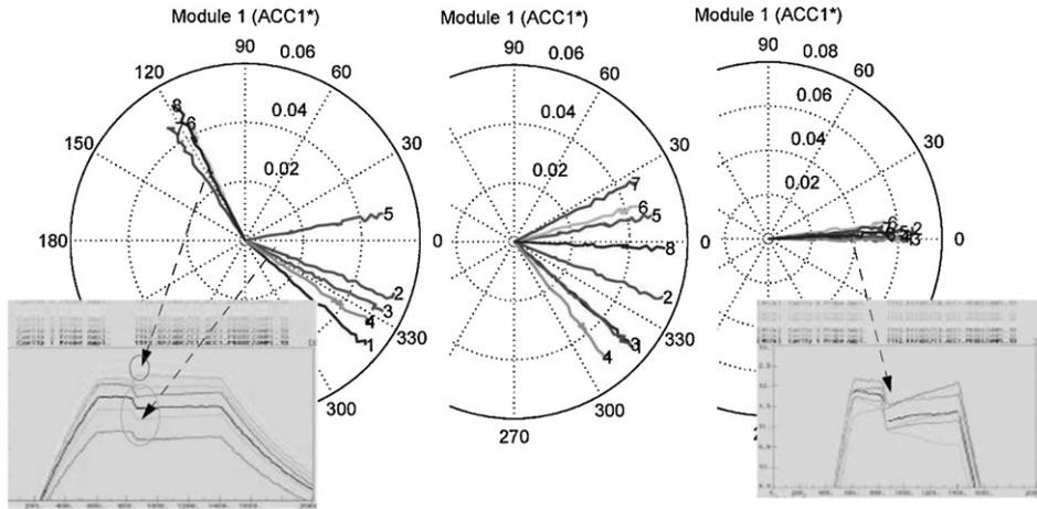
**Figure 7.** Transient detection applied to the adjustment of the incident phase. The transient portion is shown in the polar plots which show the result of the progressive tuning of the incident phase from left to right.
