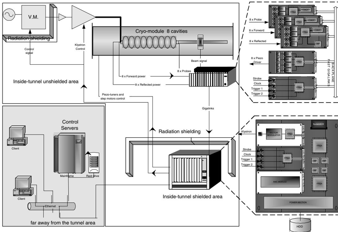
Figure 2. Hardware architecture of the RF system.
