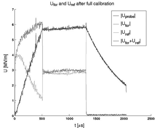
Figure 4. Measurement of the amplitudes of probe signal, forward power and reflected power.
