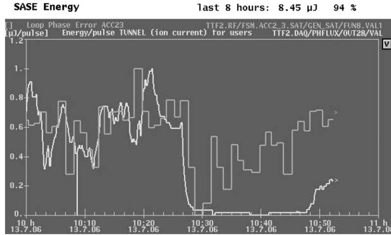
Figure 5. Measurement of loop phase and correlation with the SASE intensity
