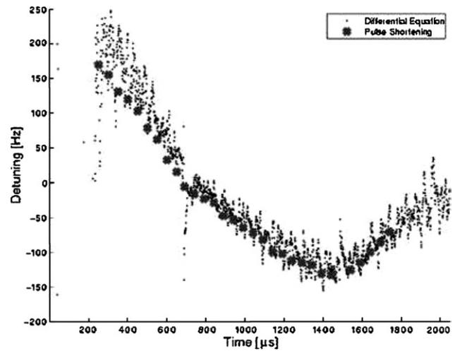
Figure 6. Cavity detuning measurement solving the differential equation and with pulse length scan where the detuning is measured at the beginning of the field decay.
