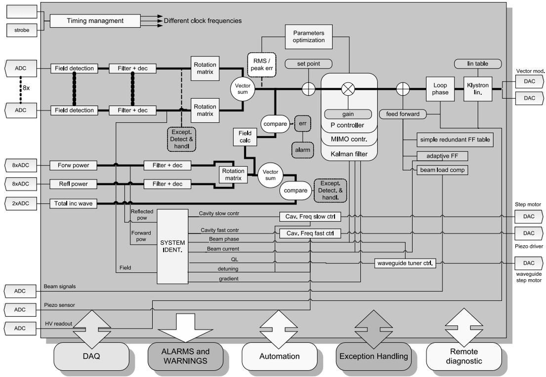
Figure 3. Software architecture and signal flow.
